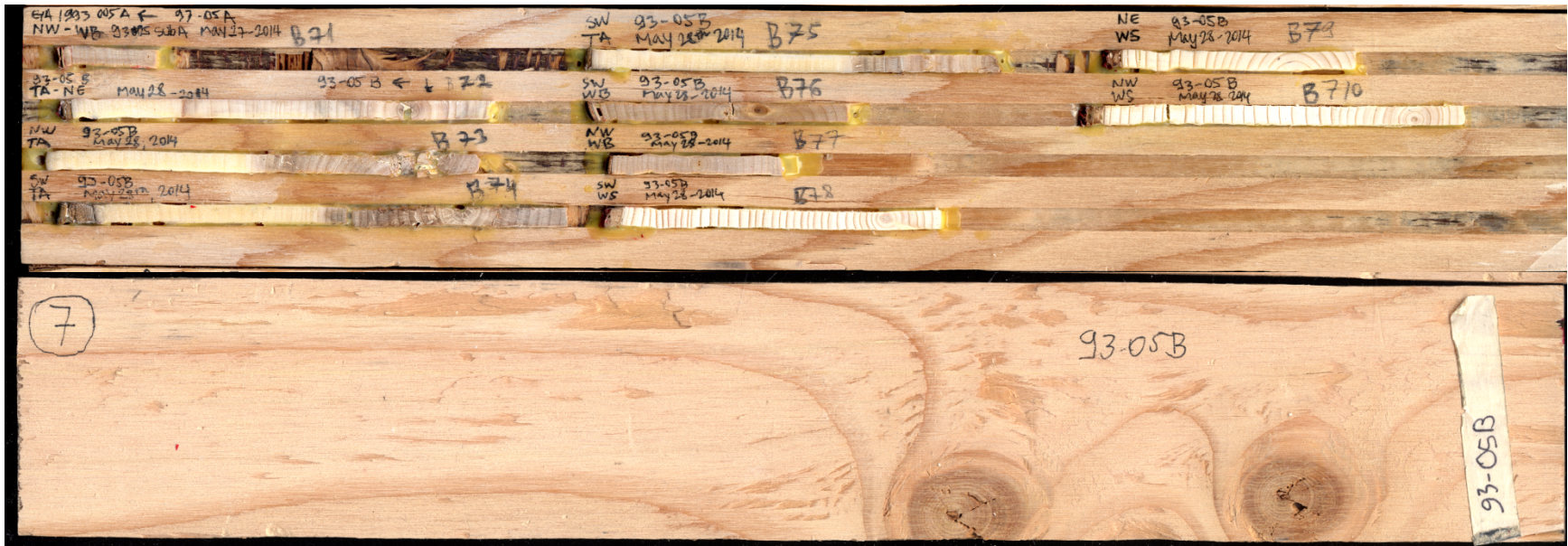
Board 7 – Front showing the cores and back showing the plots information and board number.
