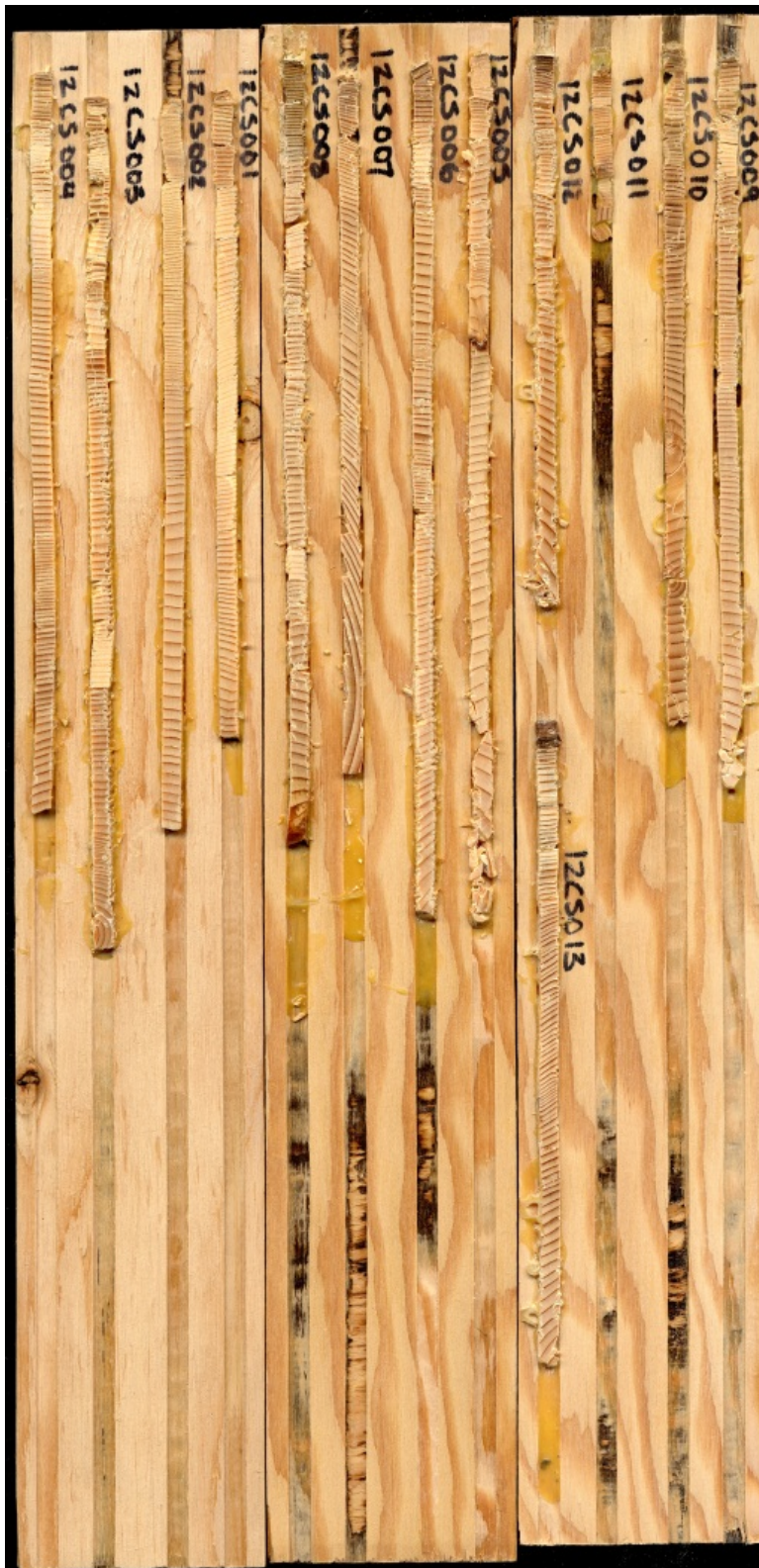
Figure 3: The thirteen samples on slotted mounting boards after sanding. Annual-growth rings are more clearly visible after sanding.
