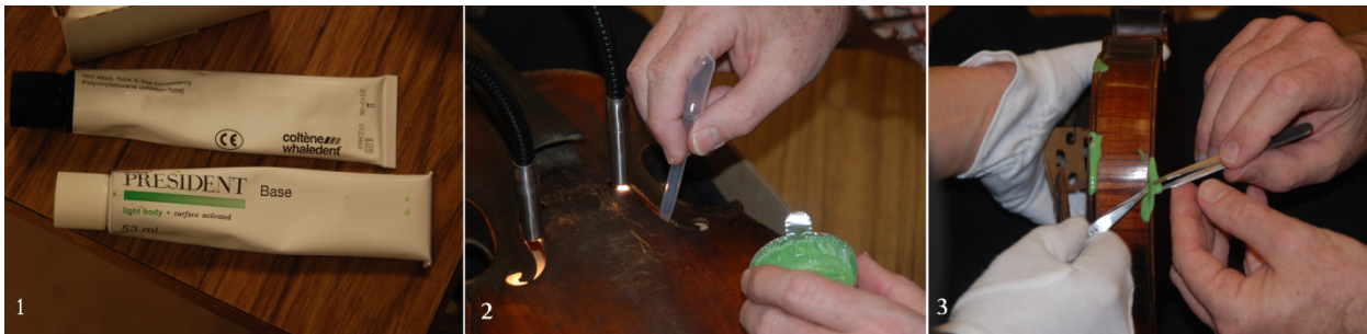
Figure 5: Taking silicone samples from the violin- 1) the base and accelerant are mixed, 2) pipetting the mixture into the violin while it is still in a liquid state, 3) removing the hardened silicone cast after it has hardened.
