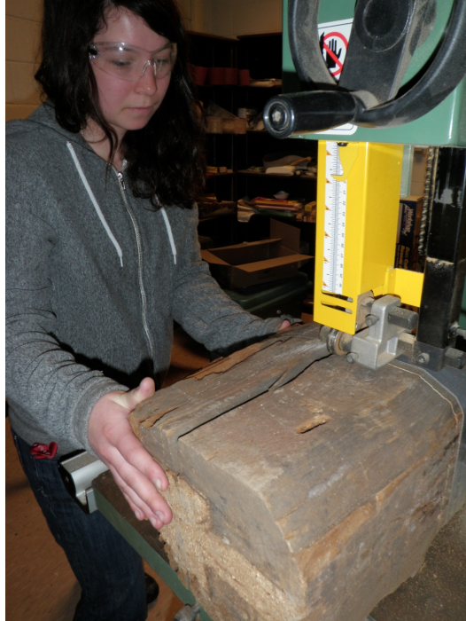
Figure 2: Utilizing the band saw to cut out disk samples.
