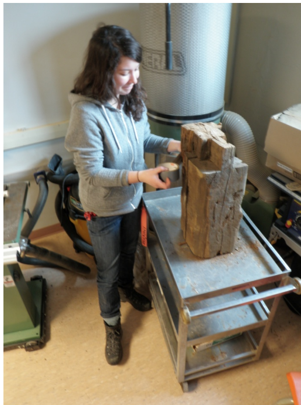
Figure 1. Taping up samples in order to cut out disks. Areas of the sample that contained perimeter wood edges were selected to be used.
