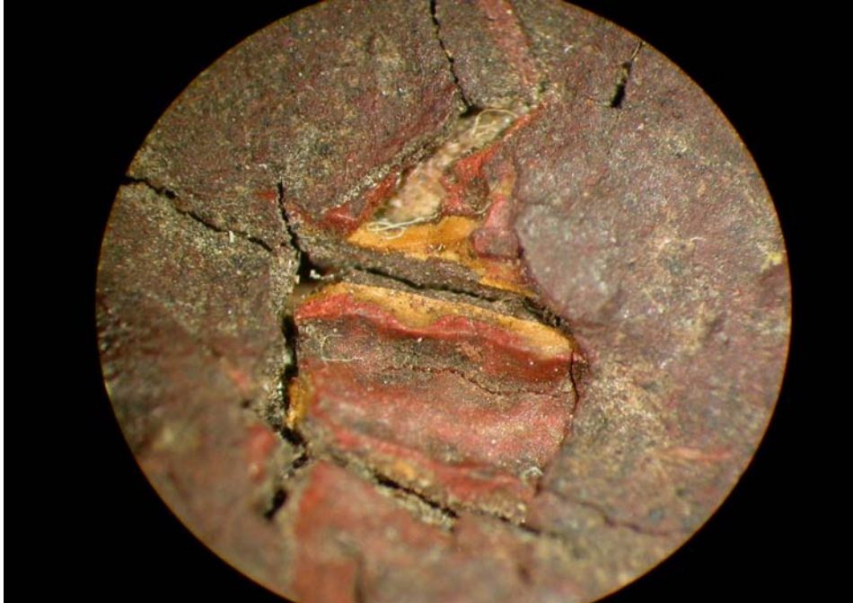
Figure 7. An example of an area of the stick surface under high magnification. Cracked and chipped pieces of the paint and varnish layers are clearly visible. In this image, four different layers demarcated by colour can be distinguished.
