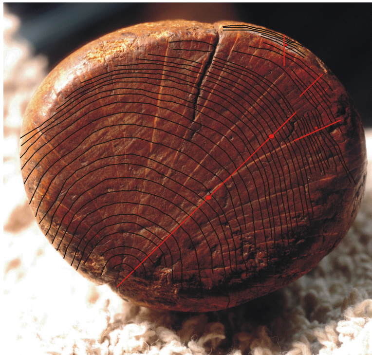
Figure 3. The red line indicates the direction of the second independent path sampled and measured. Overall rings patterns were drawn on the butt in the black lines on the stick in a graphics program.
