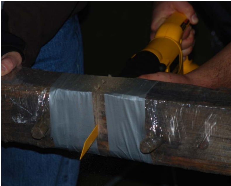
Figure 3. Sampling the cross-beam of the Basque boat with a reciprocating saw.
